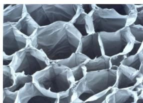
Photomicrograph of internal Structure of Broadleaf P4 water-storing polymer showing honeycomb water-holding formation
